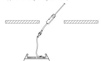
9 Push up spring-arms on side of fixture, lift into ceiling, and release spring-arms.
